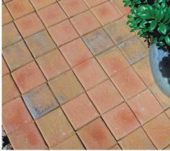
The Coleford Cobble Paver has been designed to recreate an individual  $100 \, x$   $100 \, \text{mm}$  cobble. To make the handling and laying process as efficient as possible two  $100 \, \text{mm}$  cobbles have been linked together to form a profiled paver. To increase the laying patterns available, the centre channel in the paver can be used as a cutting guide to create single cobbles.
